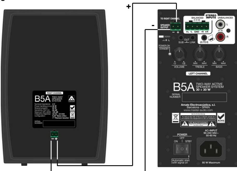
Fig.5. Connection from active speaker to passive speaker
